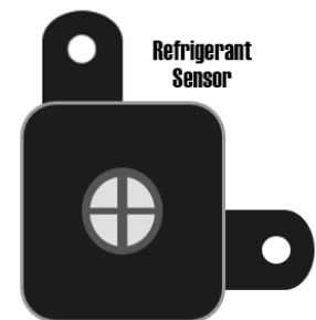
Figure 1: RDS intended for high probability systems for human comfort will typically consist of a control board to output the signal, and one or more sensors to detect the refrigerant.
