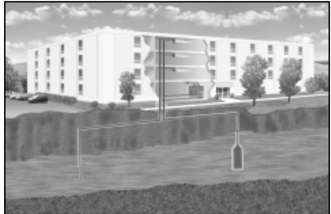
Open Loop Well Application
