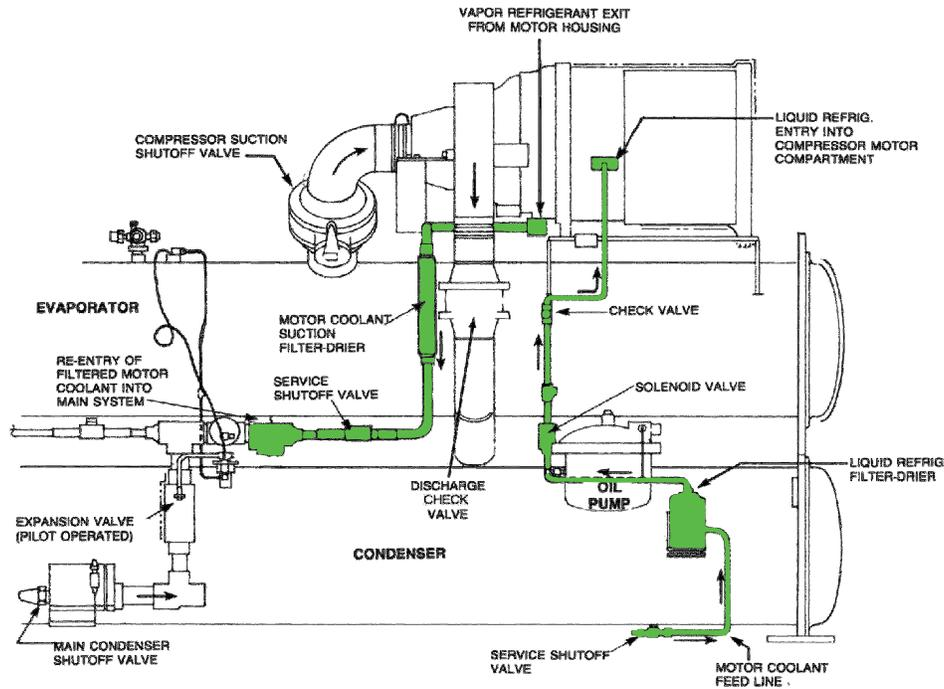
Over 30 years of field experience have proven the reliability of these compressor motors. Despite the reliability inherent in the motor design and the protective control, electrical distribution system faults and lightning strikes can occur that are beyond the control of the most conscientious designer. The coolant protective system protects the unit charge from being contaminated.
