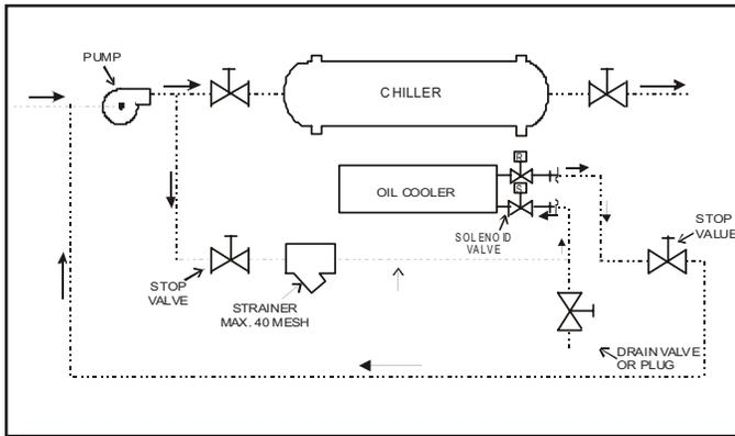
**Figure 14: WDC/WCC Oil Cooler Piping With City Water**
