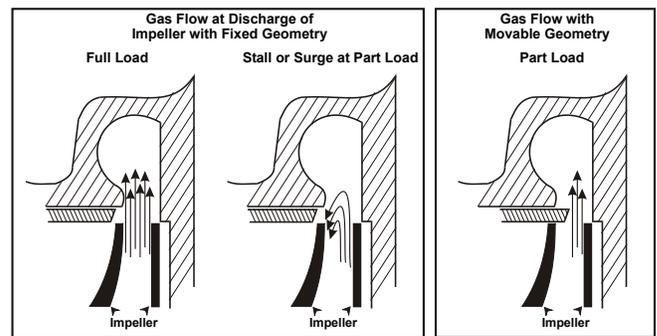
Figure 1 shows a cross-section view of the operation at full load of a unit with a fixed compressor discharge. At full load, a large quantity of gas is discharged with a fairly uniform discharge velocity as indicated by the arrows.
