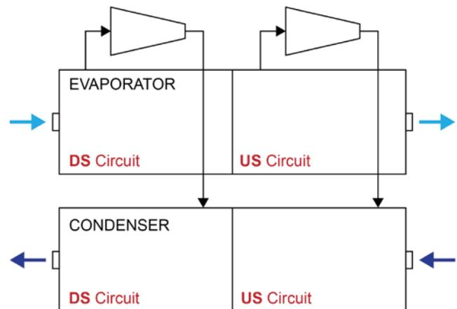
Dual circuit WCC series counterflow chillers have a separate refrigerant circuit for each compressor. They are available in single pass only. By reducing the lift on each compressor, they provide the high full load efficiency advantage of two separate chillers arranged for counterflow operation in a single, compact unit.
