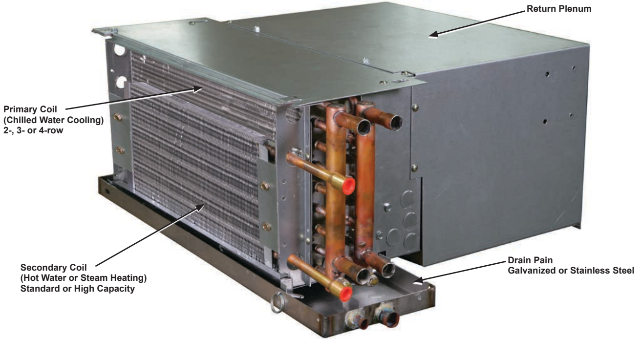
Figure 3: Model FCHH with Return Plenum Features
