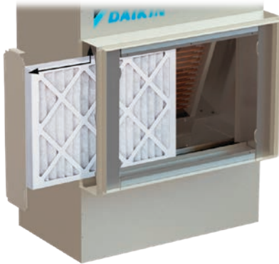
Figure 10: Unit Sizes 006 - 020 External Filter Removal on Left Side
