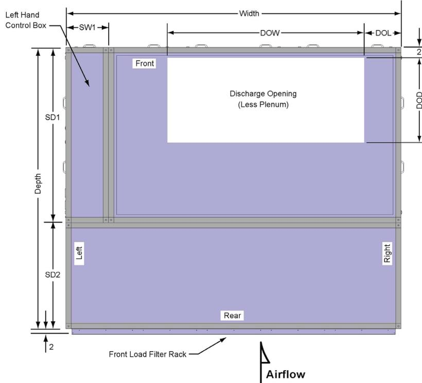
Figure 60: SWP Discharge Plenum Dimensions
