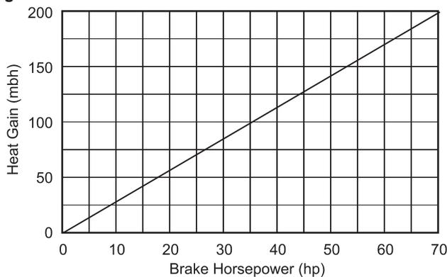
$$\text{Fan temperature rise} = \frac{(\text{fan heat (MBh)})}{(1.085 \times \text{fan cfm})}$$
