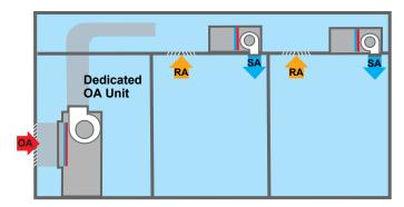
Delivered to the supply ductwork from the space unit (Figure 15). This method mixes ventilation air with the local unit supply airflow. Balancing can be difficult due to the positive pressure of the supply ductwork.
