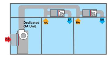
• Delivered to the return plenum for the space unit (Figure 14). This method mixes ventilation air with return air in the plenum. Because the ventilation air distribution is not directly connected to the space airflow distribution it is difficult to ensure the required ventilation airflow reaches the occupied zone. ASHRAE 62.1 provides guidance on using this distribution method and should be referenced for additional information. Local codes should also be reviewed.
