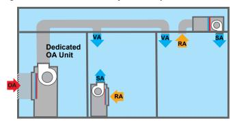
Delivered to the intake of the local units (Figure 13). This method uses the local unit air distribution to deliver ventilation airflow to the space, providing some first cost savings. Since the ventilation airflow is delivered directly to the local unit return air intake, the local unit fan must remain on during all occupied periods to deliver ventilation air to the space.
