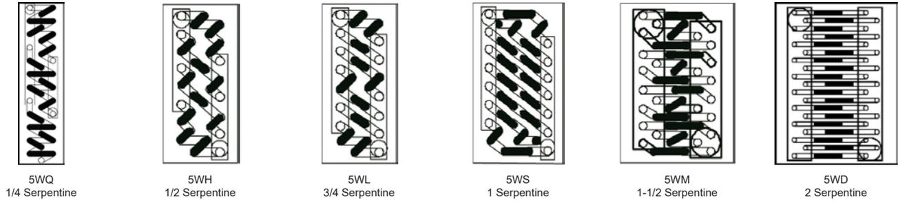
**Figure 3: Evaporator Coil Circuitings**
