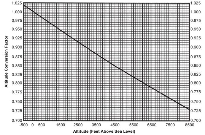
When the specified air volume (CFM) is given at any temperature other than 70° F or any altitude other than sea level, these charts should be used for correction before using the capacity and pressure drop tables which are based on CFM at standard air conditions.
