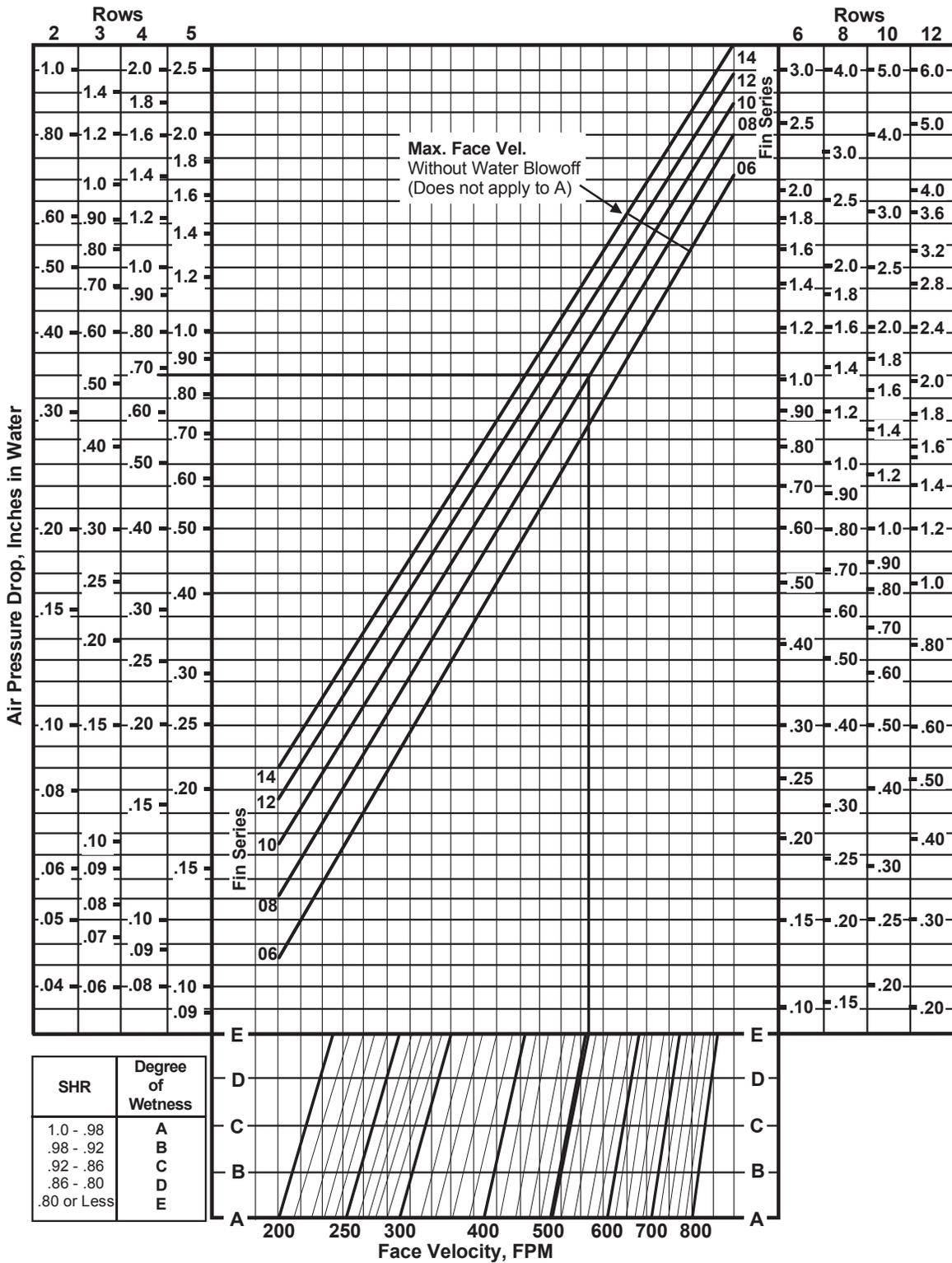
**NOTE:** The letters A, B, C, D or E indicate the degree of wetness at which the coil would be operating. Dry coils are shown by the letter A, wetcoils by the letter E. Intermediate conditions are shown by the letters B, C and D. Air pressure drop for odd fin spacings may be found by interpolation.
