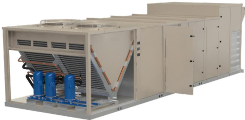
Maverick II rooftop systems are ideal for 100% dedicated outdoor air systems (DOAS). Units can be equipped with modulating hot gas reheat to increase occupant comfort and avoid over-cooling and units can incorporate an optional energy recovery wheel that can drastically improve operational costs. Also available is a 100° temperature-rise furnace for unit operation in cold-weather climates.
