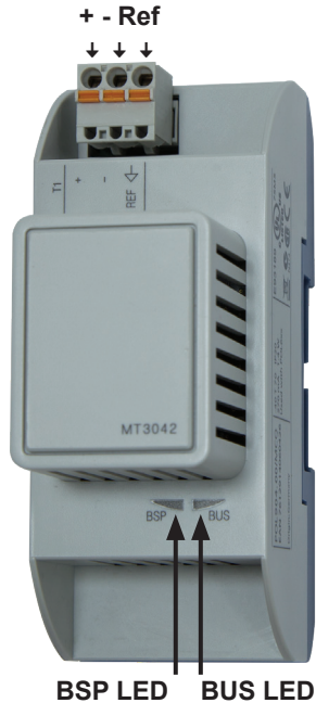
Figure 4: BACnet MS/TP Communication Module - Main Features
