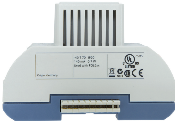
Figure 9: Communication Module with Board-to-Board Connector Inserted
