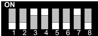
Figure 6: BACnet Communication Module Address Switch (S3) - Example of a Manual Network Address Setting
