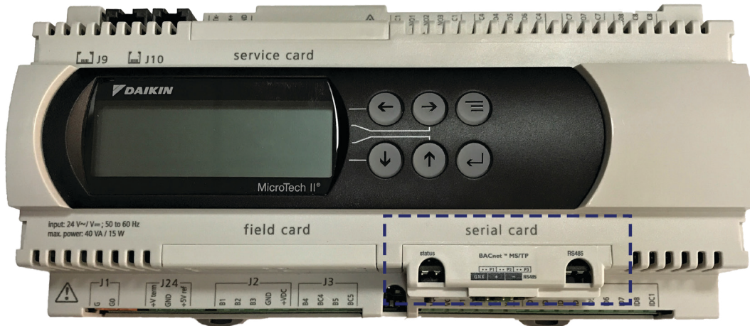
Figure 2: Current Version of BACnet MS/TP Hardware
