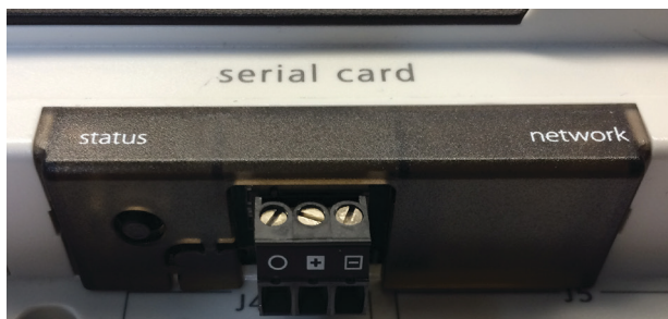
Figure 12: BACnet MS/TP Communication Module with Cover (Current Hardware)
