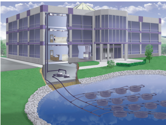
Figure 33: Surface Water Loop Application
