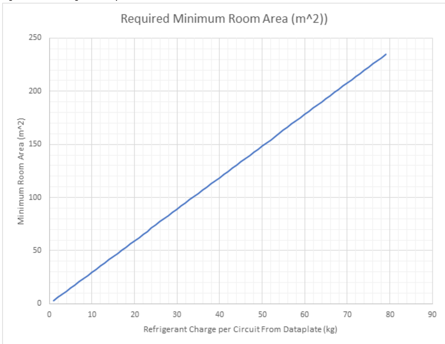
Figure 19: R-32 Refrigerant - Required Minimum Room Area Chart
