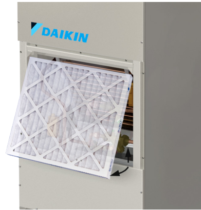
Figure 13: Unit Sizes 006 - 020 Internal Filter Removal
