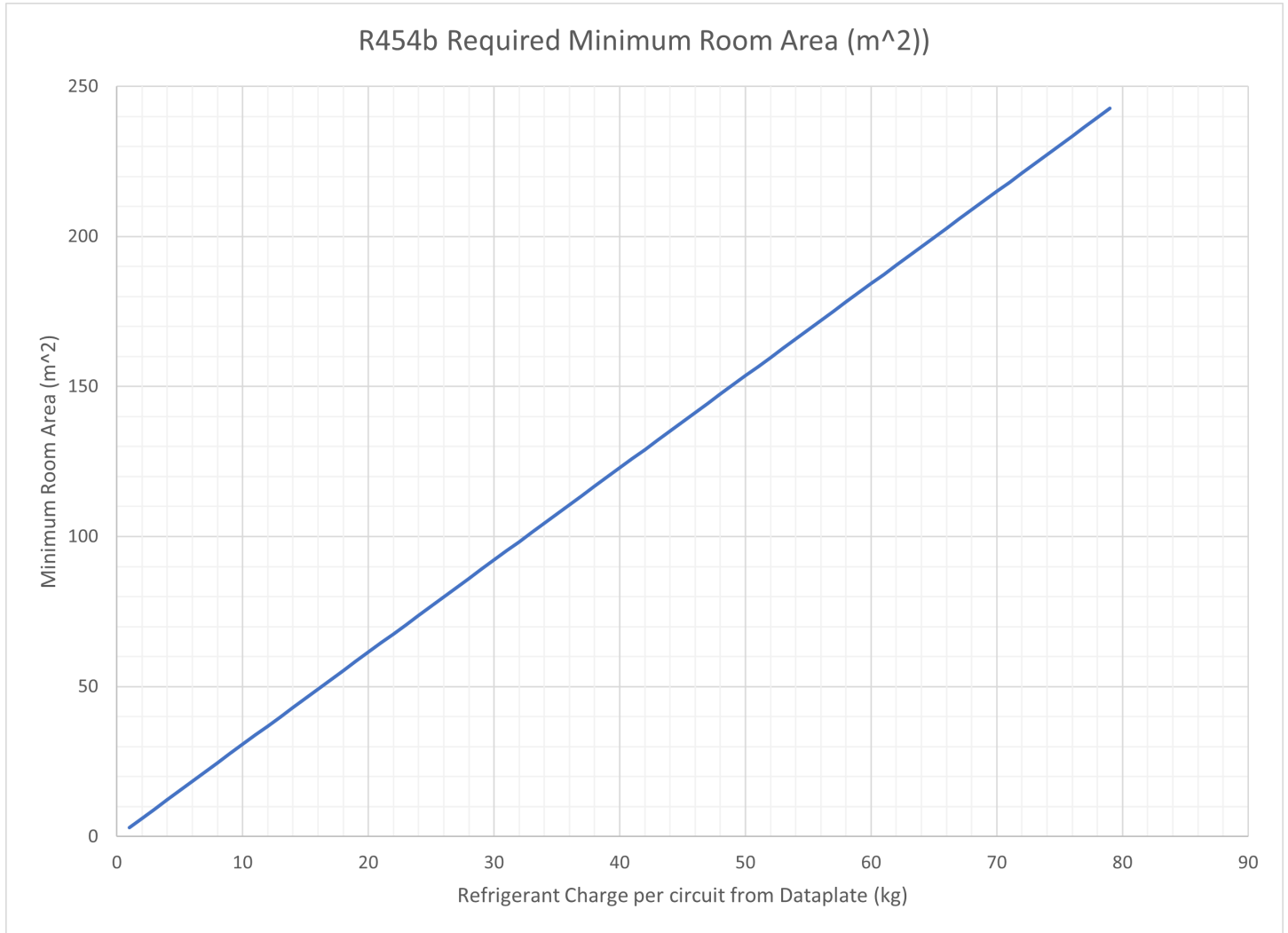
Figure 22: R-454B Refrigerant - Required Minimum Room Area Chart
