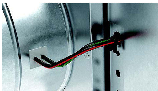
Figure 35: Inlet Flow Sensor Ports
