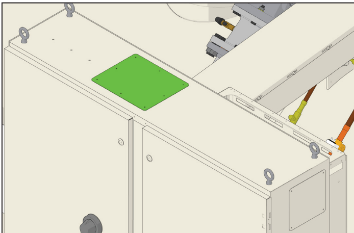
Figure 4: Unit Power Connection Point
