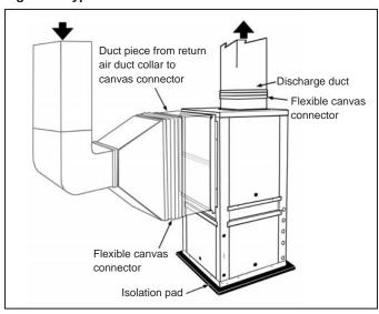
Figure 6: Vertical Unit - Typical Installation in Small Mechanical Room or Closet
