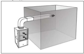
Another common configuration has the water source heat pump unit located in a mechanical closet adjacent to the occupied space. A measure of the sound levels inside the mechanical space can be best determined using the free inlet combined with the casing radiated configuration. The test setup for this is shown in Figure 3.
