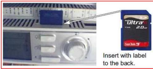
4. Save the existing configuration and parameters to the memory card.
