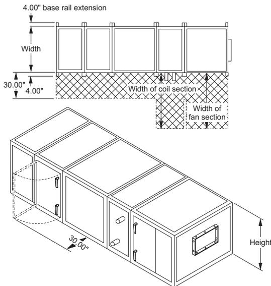
**Figure 2: Service Clearance for Electrical Power Devices**
