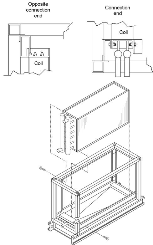
**Figure 103: Single Coil Side Installation/Removal**
