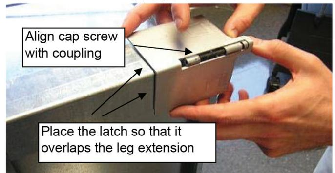
**Figure 25: Tighten Cap Screw to 1/4" of the Coupling**
