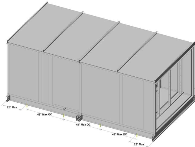
**Figure 55: Unit with Base Frame Welded**
