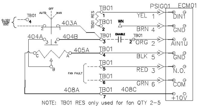
Figure 79: EBM Gen 3 Motor - Control Wiring with Manual/ Auto (Basic) Controls
