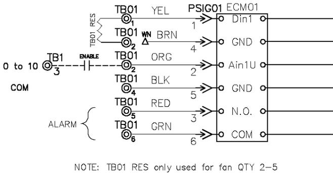
Figure 78: EBM Gen 3 Motor - Control Wiring with No Controls
