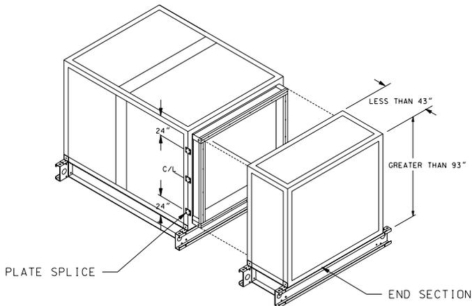
**Figure 11: Splice Collar Alignment**
