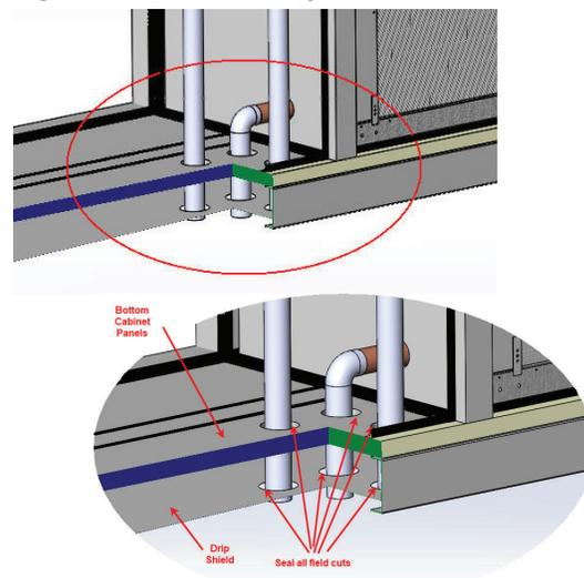
**Figure 47: Piping Arrangements**
