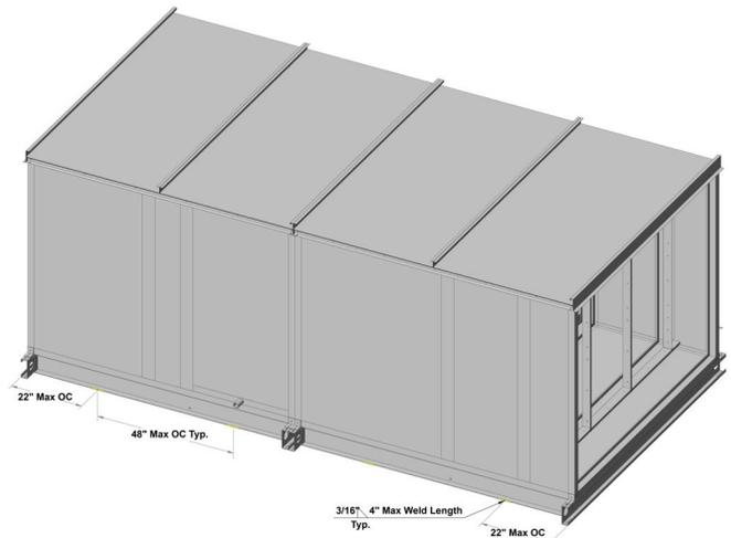
**Figure 56: Unit with Base Frame Mounted on Concrete**
