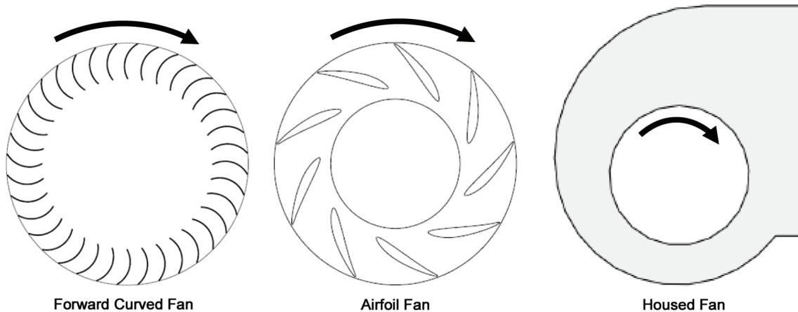
Fan wheel should rotate as shown
