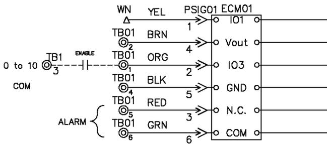
Figure 82: Delta Motor - Control Wiring with Manual/Auto (Basic) Controls
