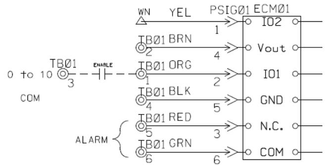
Figure 76: EBM Gen 2 Motor - Control Wiring with Manual/ Auto (Basic) Controls
