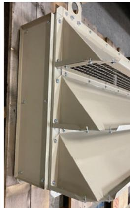
**Figure 89: Showing what a removed side panel looks like, with gaskets on inside**
