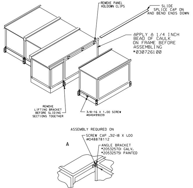
Figure 7: Apply Sealant to Mating Faces
