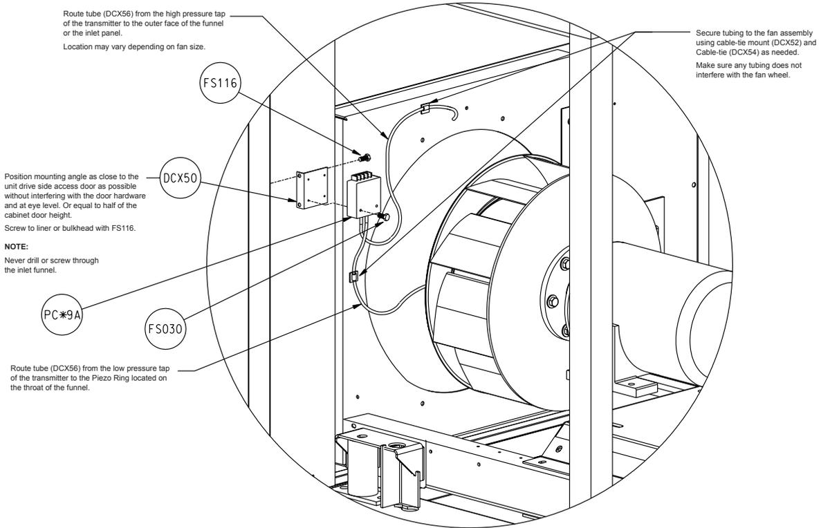
**Figure 67: Fan Array Installation**
