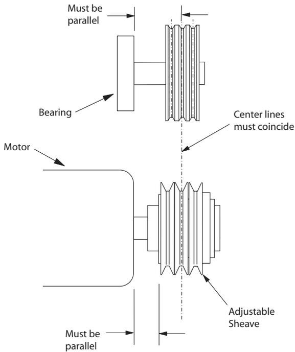
**Figure 98: Adjustable Sheave Components**
