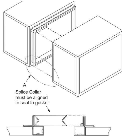
**Figure 12: D-Gasket Placement Detail (High Pressure Low Leakage Units Only)**
