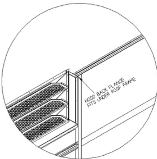
**Figure 92: Final installation**
