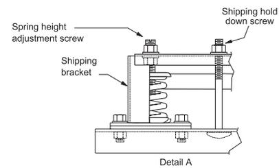
**Figure 53: Plenum Fan Typical Shipping Brackets**
