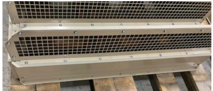
**Figure 88: Side panel of hood (one on both sides) needed to be removed to secure hood**
