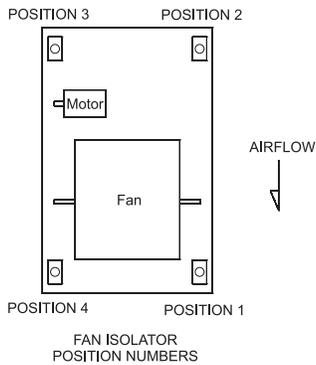
**Figure 52: Removing "Motor Beside" Shipping Brackets**
