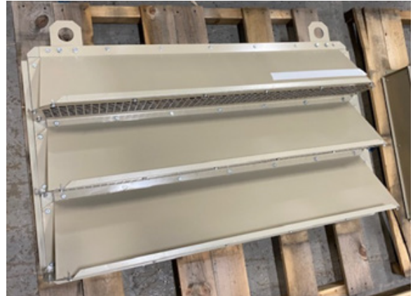
Figure 92: Top flange of hood screwed to the unit while held in place by lifting mechanism
