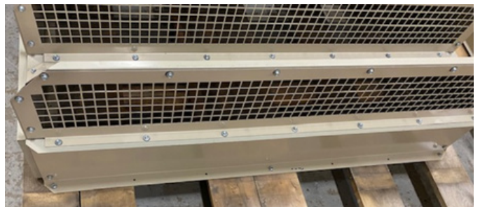
Figure 93: Bottom flange of hood screwed to unit while held in place by lifting bracket
