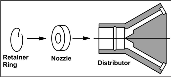
Figure 3: Hot Gas Bypass Kit
