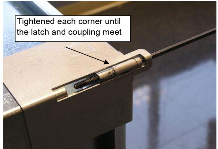
Figure 29: Properly Installed Filter Inside of the Frame
