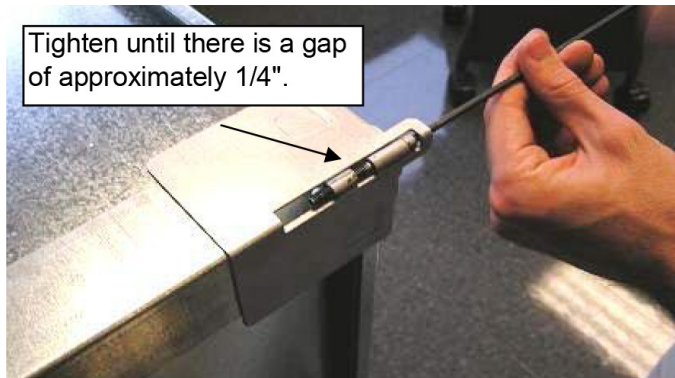
Figure 27: Tighten Cap Screw to 1/4" of the Coupling
