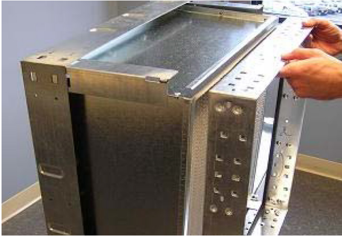
Figure 30: Positioning of the Prefilter Frame
