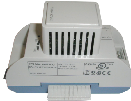
Figure 6: BACnet Communication Module with Board-to-Board Connector Inserted
