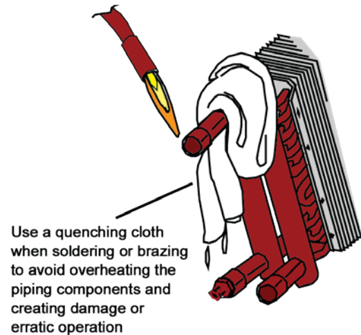
Figure 7: Protect Components From Overheating
