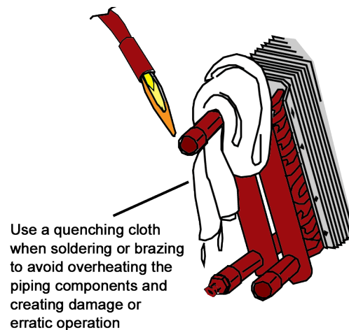
Figure 5: Protect Components from Overheating
