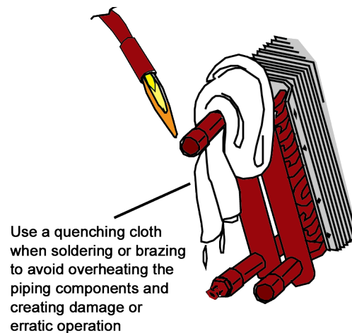
Figure 5: Protect Components from Overheating
