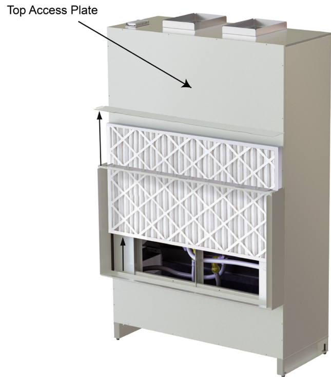
Figure 35: Top Access filter Removal (Sizes 006-020 Vertical)
