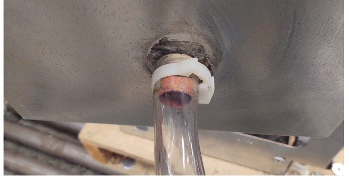
Figure 3: Connect PVC drain hose and clamp
