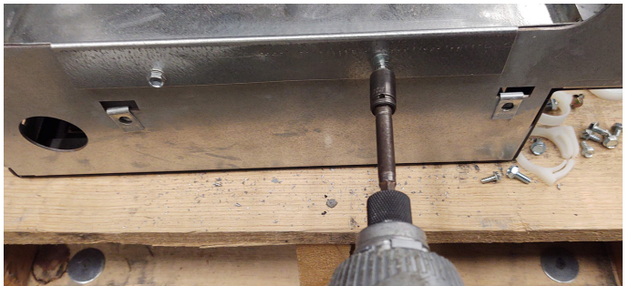
Figure 5: Secure pan to UV with provided screws
