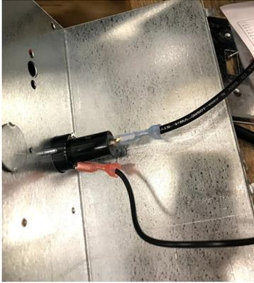
**Figure 22: Fused Power from SW1 Tying Into Red Wire (500)**
