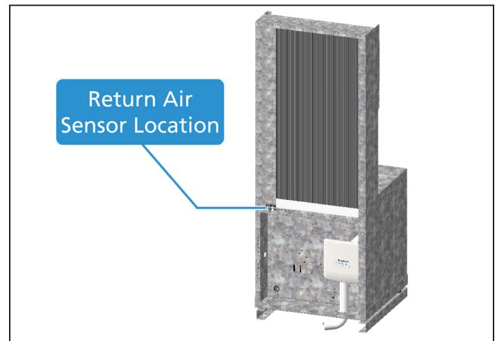
Figure 52: Return Air Temperature Sensor Location
