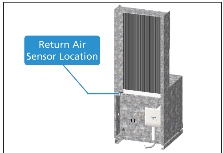
Figure 49: Return Air Temperature Sensor Location
