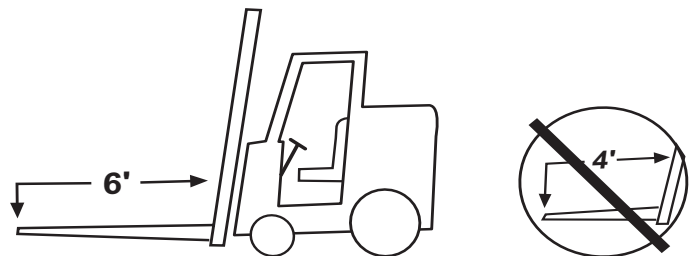
Figure 1: Forklift Lifting Requirements
