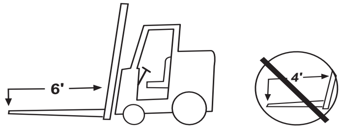
Figure 1: Forklift Lifting Requirements
