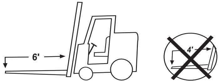
Figure 1: Forklift Lifting Requirements
