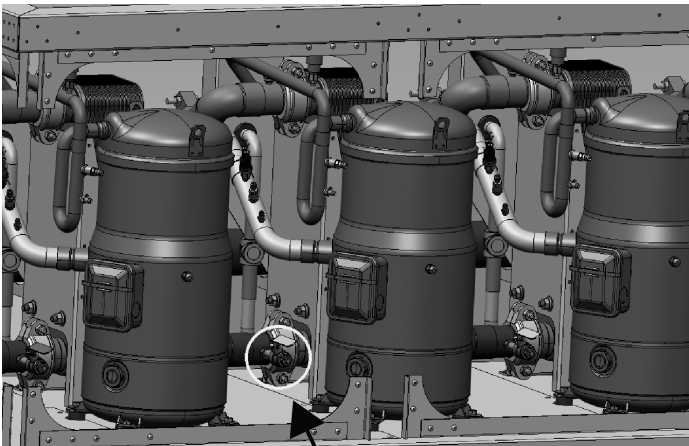
Figure 28: Condenser Water Supply Drain Valve
