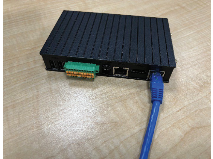
Figure 27: SiteLine Gateway ETH1 Connection
