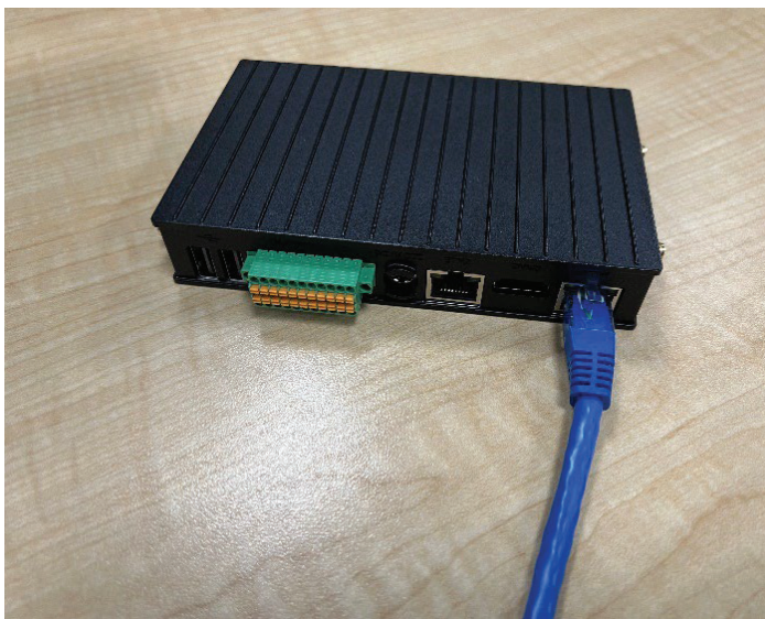
Figure 67: SiteLine Gateway ETH1 Connection
