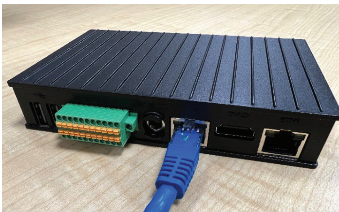
Figure 15: SiteLine Gateway ETH2 Connection
