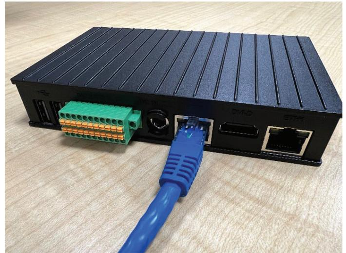
**Figure 59: Tip Port Connection (MicroTech 4 shown)**
