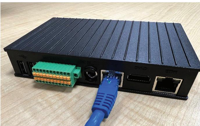
Figure 16: TIP Port Connection (MicroTech 4 shown)
