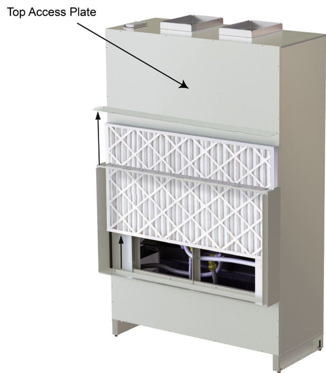
Figure 55: Top Access filter Removal (Sizes 006-020 Vertical)
