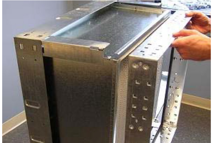
Figure 49: Positioning of the Prefilter Frame
