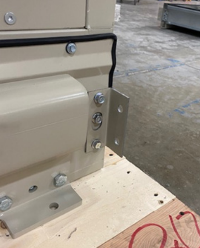
Figure 100: Lifting lugs located on base rail
