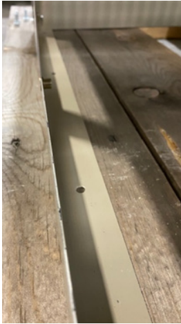
Figure 96: Side flange to be secured once side panel is removed
