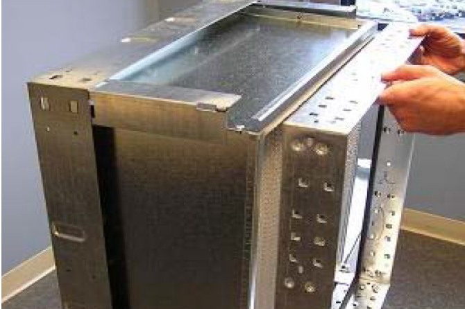
Figure 31: Positioning of the prefilter frame
