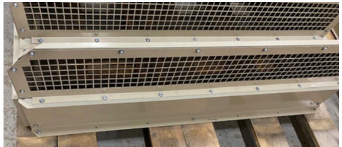
Figure 94: Side panel of hood (one on both sides) needed to be removed to secure hood
