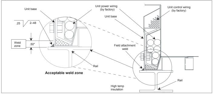
Figure 5: Weld locations for rail arrangement
