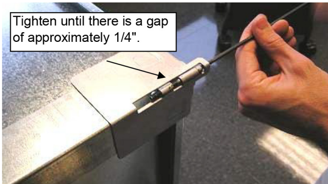
Figure 27: Tighten Cap Screw to 1/4" of the Coupling
