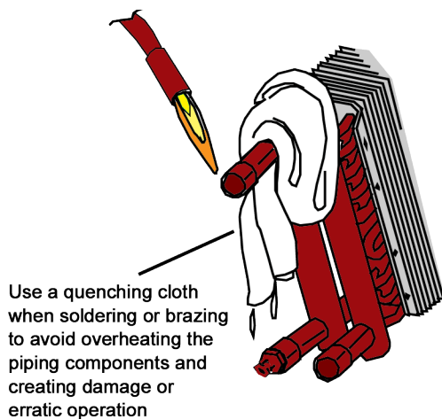
Figure 6: Protect Components from Overheating
