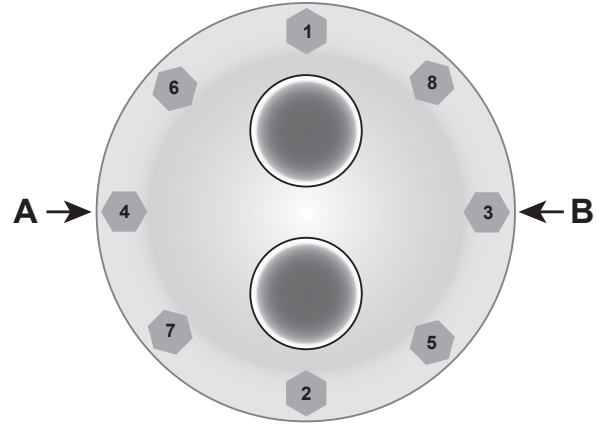
Figure 31: Centering pin location and bolt order
