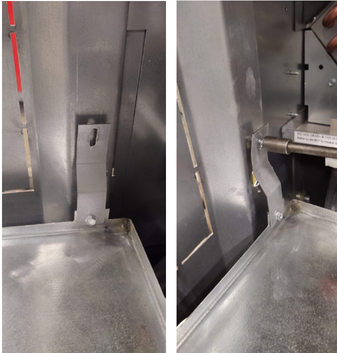
Figure 6: Attach strap to rear of unit (do not tighten)
