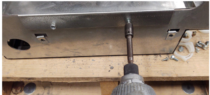
Figure 5: Secure pan to UV with provided screws
