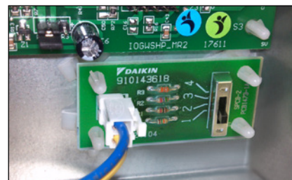
Figure 26: 4-Position Fan Speed Selector Switch
