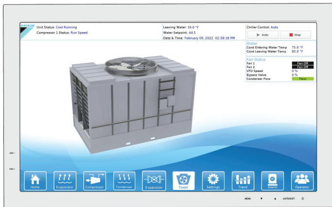
Figure 37: Cooling Tower Information
