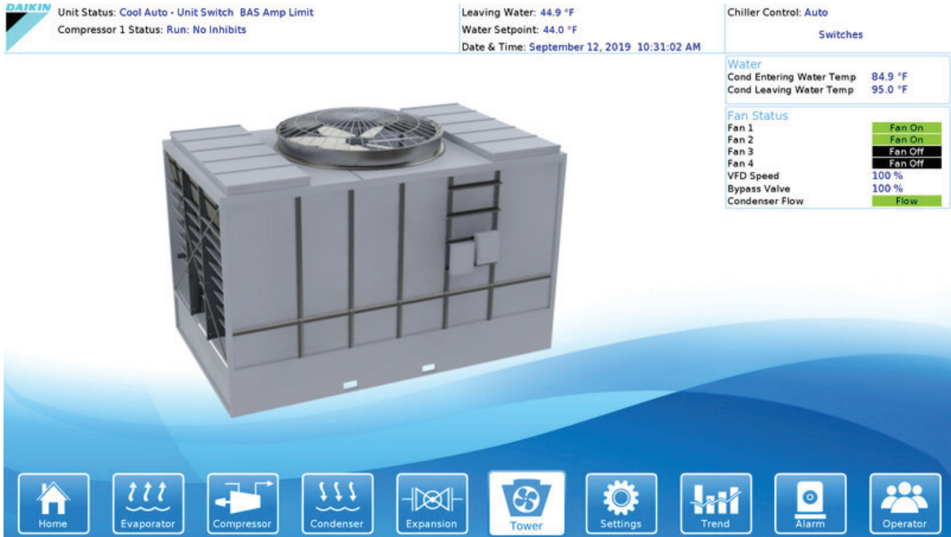
Figure 50: Cooling Tower Information
